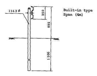
Fig. 7-7 Road sign and guard rail
