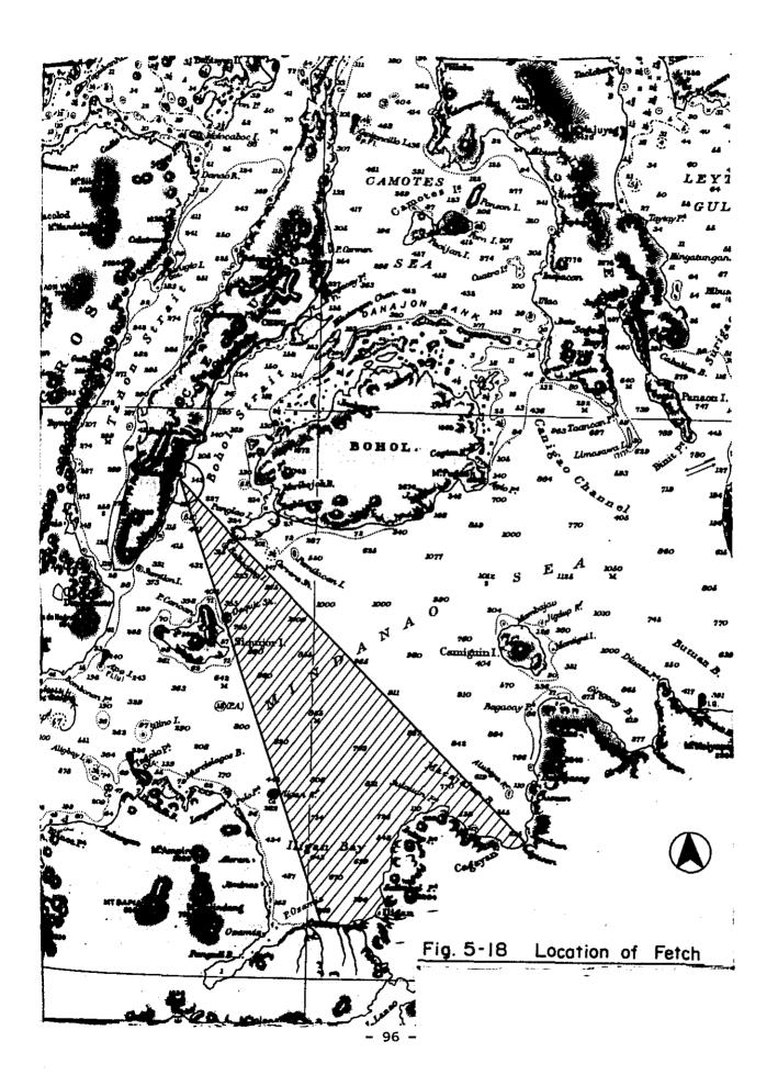
Figure 5-17 shows the oceanic distribution of wind velocity and, theoretically, a typhoon must pass over Mindanao Island to arrive at the projected area. In general, it is said that wind that pases overland loses its velocity by 30 to 40% and consideration is given to this respect in the present calculation. It is to be noted, however, that such waves are less likely to occur. On the other hand, wave calculation is made on the biannual typhoon (with average wind velocity of 15m/sec.) as follows.
