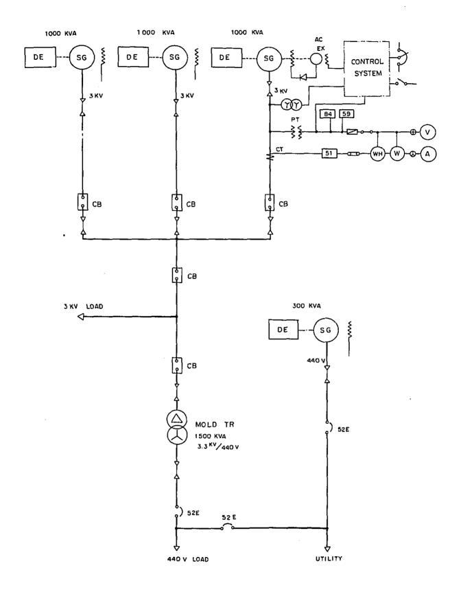
Fig. 6-5 One line Diagram of Power Station, 3KV, 3MVA
