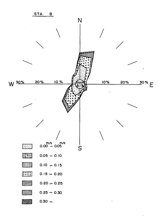
Fig. 5-9 Directions and Velocities Frequency Distribution of the Tidal Currents
