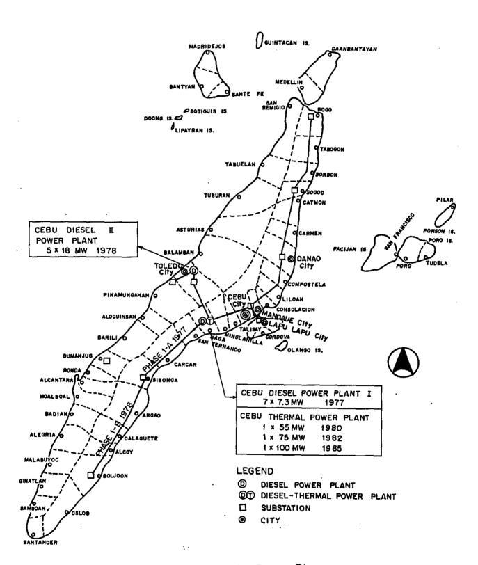
Fig. 6-1 CEBU Electric Power Plan
