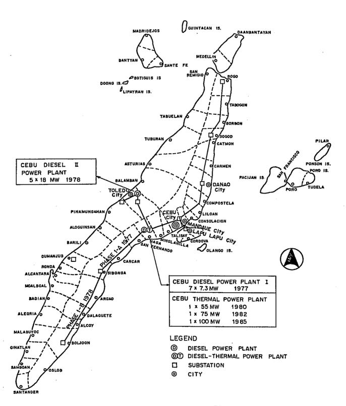
Fig. 1 - 3 CEBU Electric Power Plan
