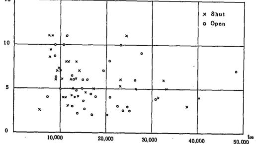
On assumption that a vessel berths itself without the aid of tug boat in the projected operation of vessel, the berthing speed of lightly loaded vessel is calculated as 30cm/sec. by the following formula. In case a vessel is loaded fully with cargo, the berthing speed is assumed 12cm/sec. on the basis of maximum value in figure 5-25 and in consideration of the rollings and shifts of a vessel.
