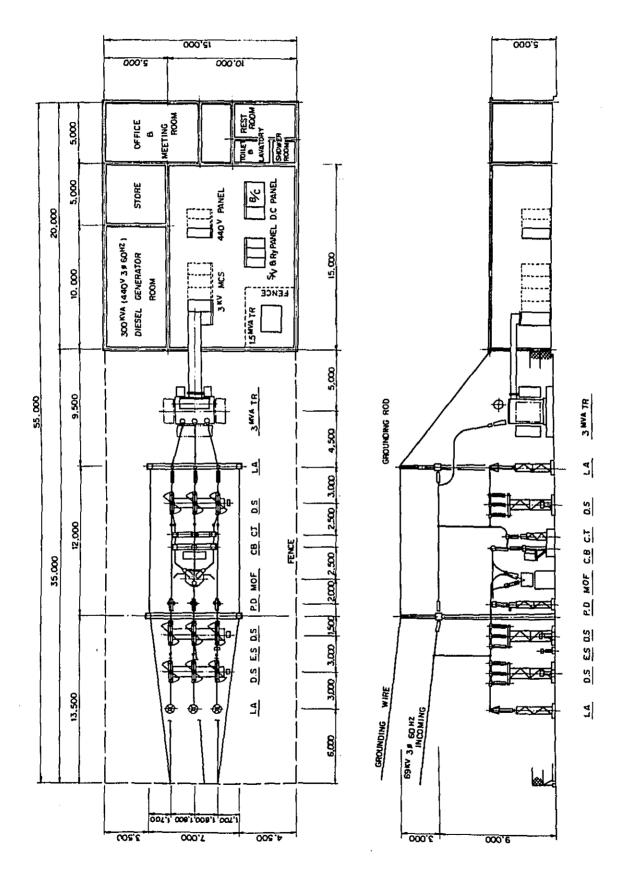
Fig. 6-4 Layout of Substation, 69KV, 3MVA
