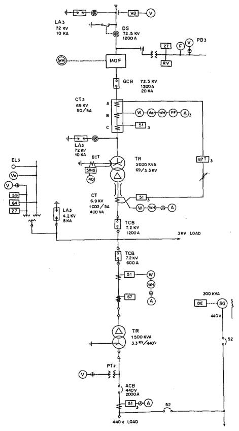
Fig. 6-3 One line Diagram of Substation 69KV, 3 MVA
