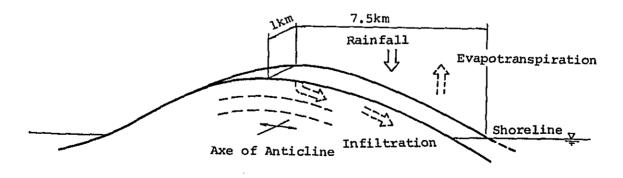
Fig. 8-4 Schematic diagram of water balance
