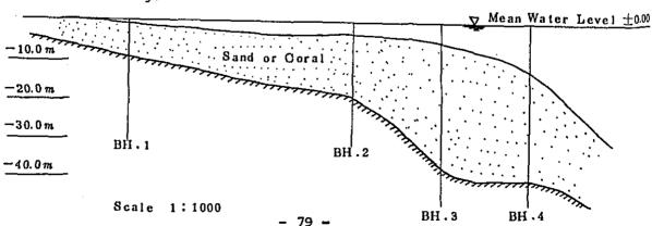
Fig. 5-2 Presumptive view of soil layer
