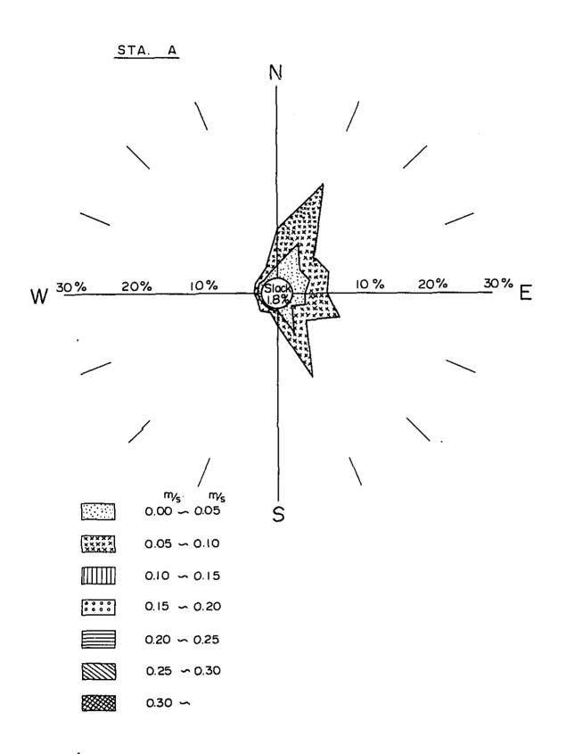
Fig. 5 - 8 Directions and Velocities Frequency Distribution of the Tidal Currents
