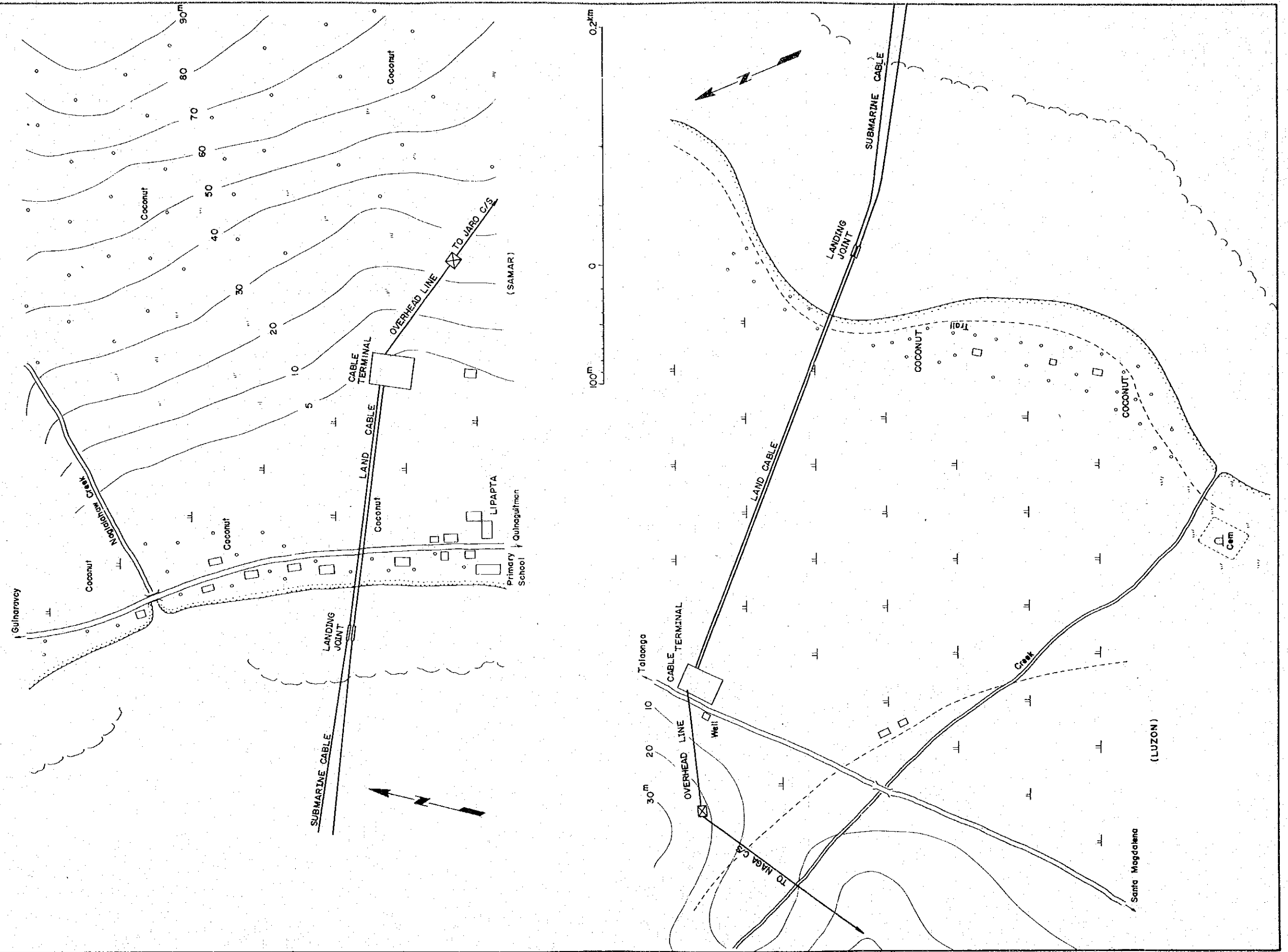
Fig.6-6 CABLE LANDING SITE AND CABLE TERMINAL SITE
