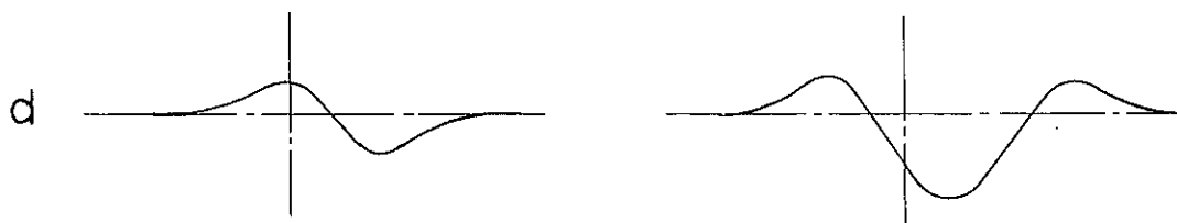
Fig. A-2-1 A Few Examples of Magnetic Anomaly Record Detected by the MB-100 Probe
