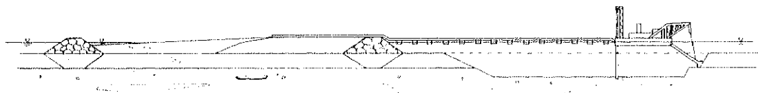
Fig. 5-1-1 Reclamation with Sand and Clayey Soil
