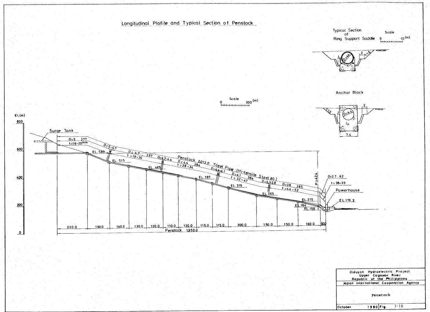
The thickness of the steel pipe plates will gradually change from 16 mm to 52 mm, according to the hydrodynamic pressure.
