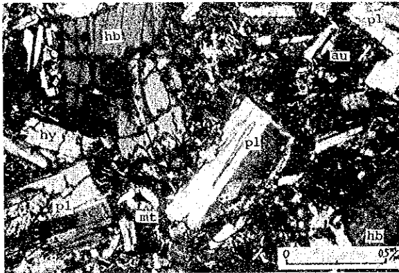
Fig. II-1-16b Microscopic Photograph of Sample no. M-46, augite-hypersthene-hornblende andesite intersertal texture
