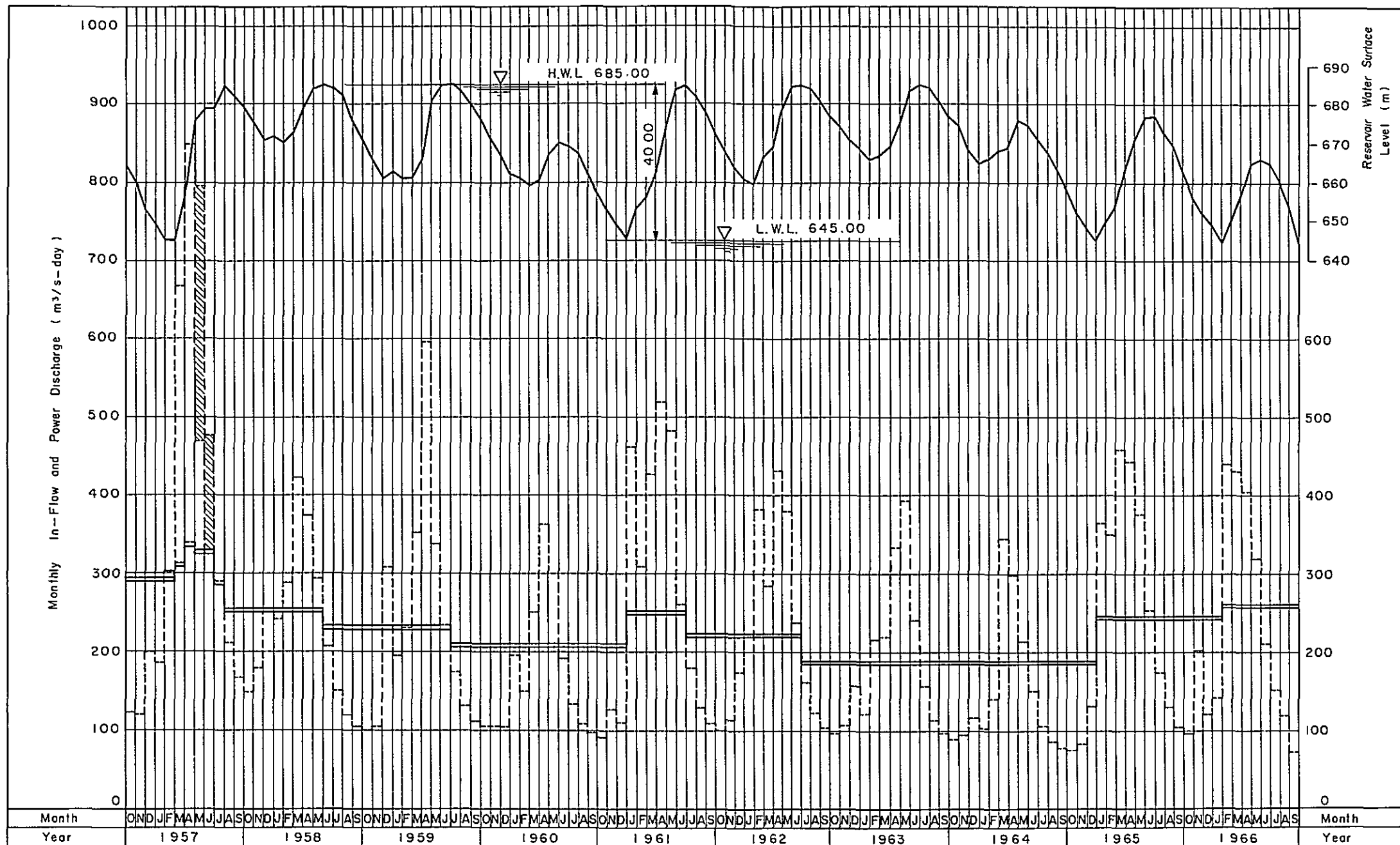
KARUN 562 RESERVOIR IN-FLOW, POWER DISCHARGE AND RESERVOIR WATER SURFACE
