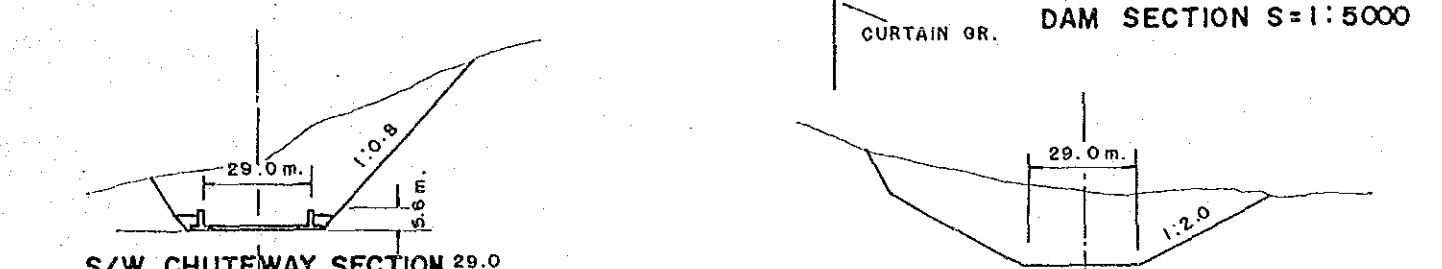
S/W CHUTEWAY SECTION S=1:2000
