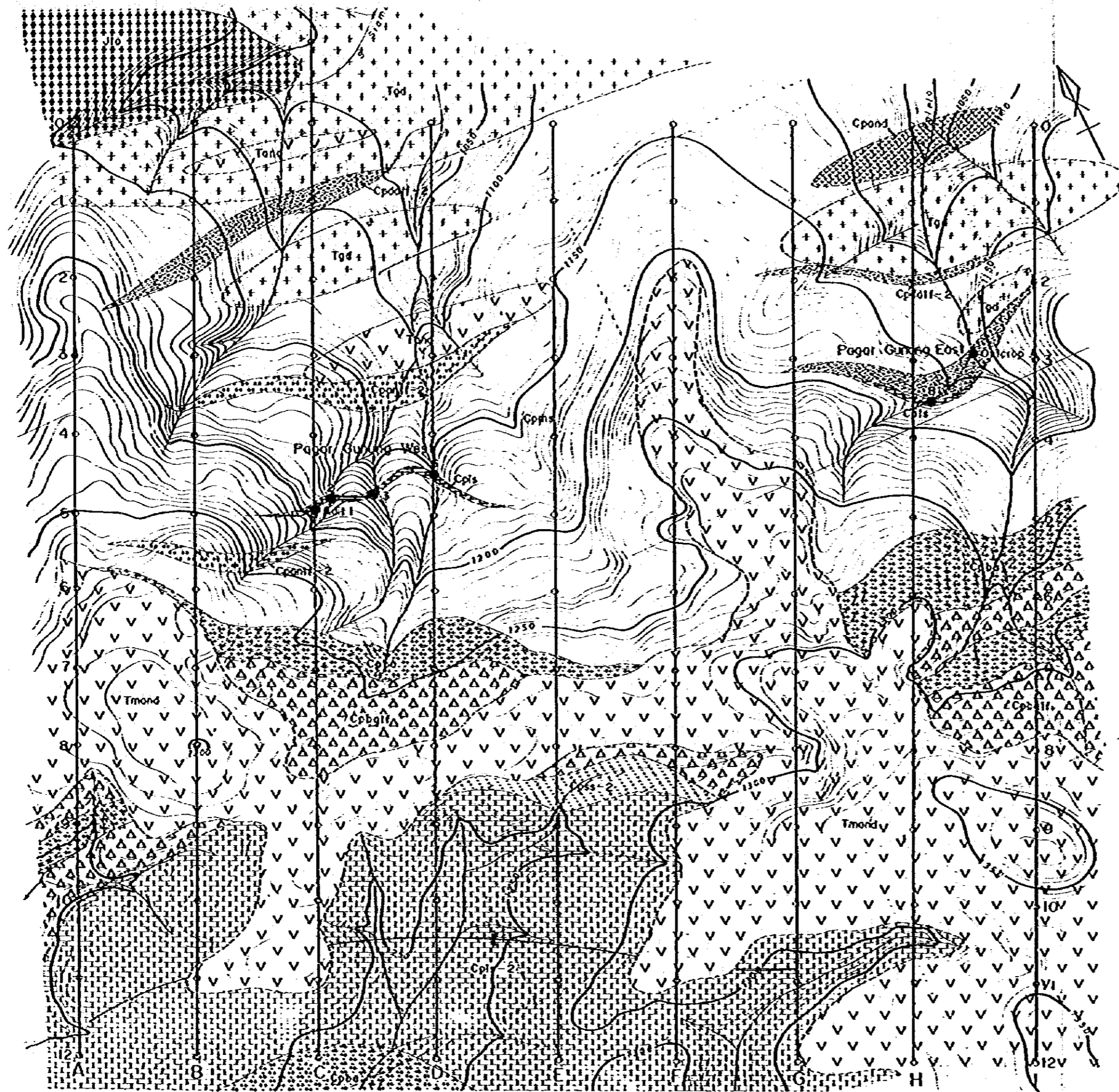
Fig. II-3-7 Geological Map of Pagar Gunung Ore Deposit Area, Huara Sipongi Area B
