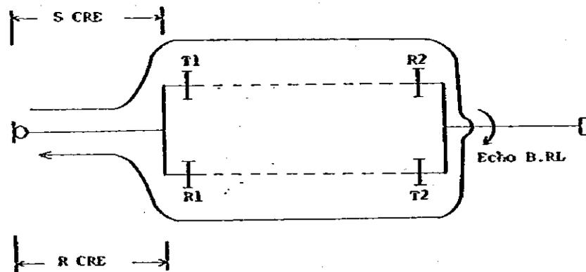
$$\text{反響経路損失} = \text{SCRE} + T_1 + R_2 + \text{Echo B.RL} + T_2 + R_1 + \text{RCRE}$$
