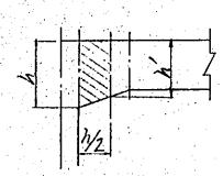
For the disign of section of beam end the value of shearing stress at 1/2 point is applied
