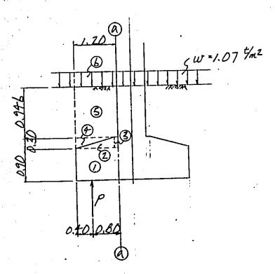
$N_1 = 2.5 \times 1.20 \times 0.90 \times 4.30 = 11.61^{t}$   $N_2 = 2.5 \times 1/2 \times 1.10 \times 0.30 \times 4.30 = 1.77^{"}$   $N_3 = 2.5 \times 0.10 \times 0.30 \times 4.30 = 0.32^{"}$   $N_4 = 1.8 \times 1/2 \times 1.10 \times 0.30 \times 4.30 = 1.28^{"}$   $N_5 = 1.8 \times 1.20 \times 0.946 \times 4.30 = 8.79^{"}$   $N_5 = 1.07 \times 1.20 \times 4.30 = 5.52^{"}$
