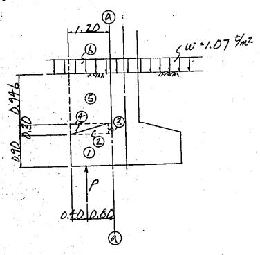
$N_1 = 2.5 \times 1.20 \times 0.90 \times 4.30 = 11.61^{t}$   $N_2 = 2.5 \times 1/2 \times 1.10 \times 0.30 \times 4.30 = 1.77^{"}$   $N_3 = 2.5 \times 0.10 \times 0.30 \times 4.30 = 0.32^{"}$   $N_4 = 1.8 \times 1/2 \times 1.10 \times 0.30 \times 4.30 = 1.28^{"}$   $N_5 = 1.8 \times 1.20 \times 0.946 \times 4.30 = 8.79^{"}$   $N_6 = 1.07 \times 1.20 \times 4.30 = 5.52^{"}$
