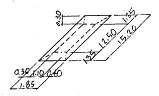
$V_{C} = \frac{0.30}{6} \times \left\{ 1.10 \times 12.50 + 1.85 \times 15.20 + (1.10 + 1.85) \times (12.50 + 15.20) \right\} =$
