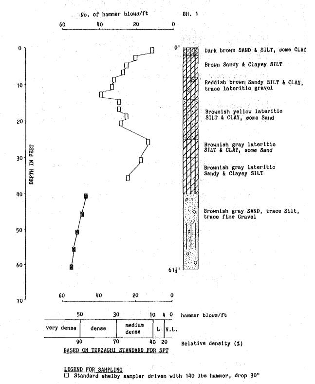
Standard split spoon sampler driven with 140 lbs hammer, drop 30"
