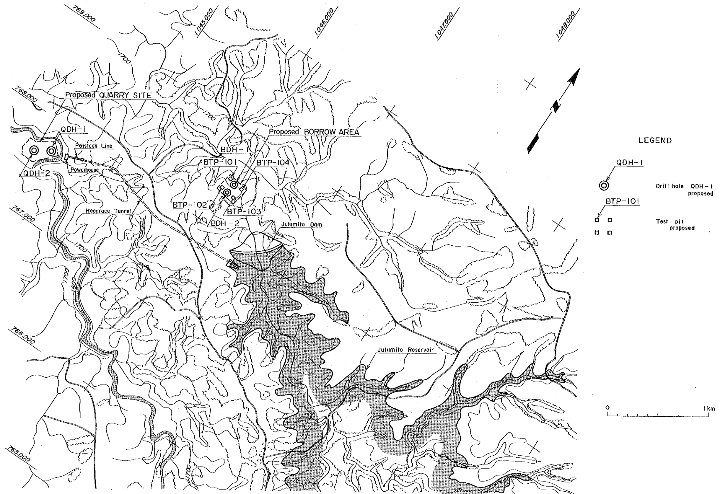
Fig. 1-9 Location Map for Recommended Geological Investigation Works at Borrow Area and Quarry Site (Plan)
