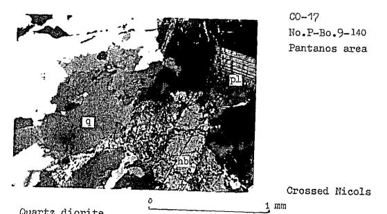
Quartz diorite Divided quartz shows wave-extinction, i.e. cataclastic structure. Chloritization and sericitization are moderately. Hornblende has changed mostly to chlorite and sphene.
