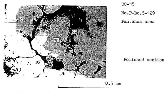
Pyrite and chalcopyrite with chalcocite rim in the quartz veinlets.
