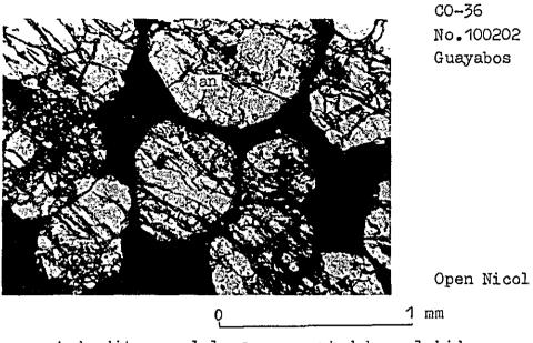
Andradite crystals are cemented by sulphide.
