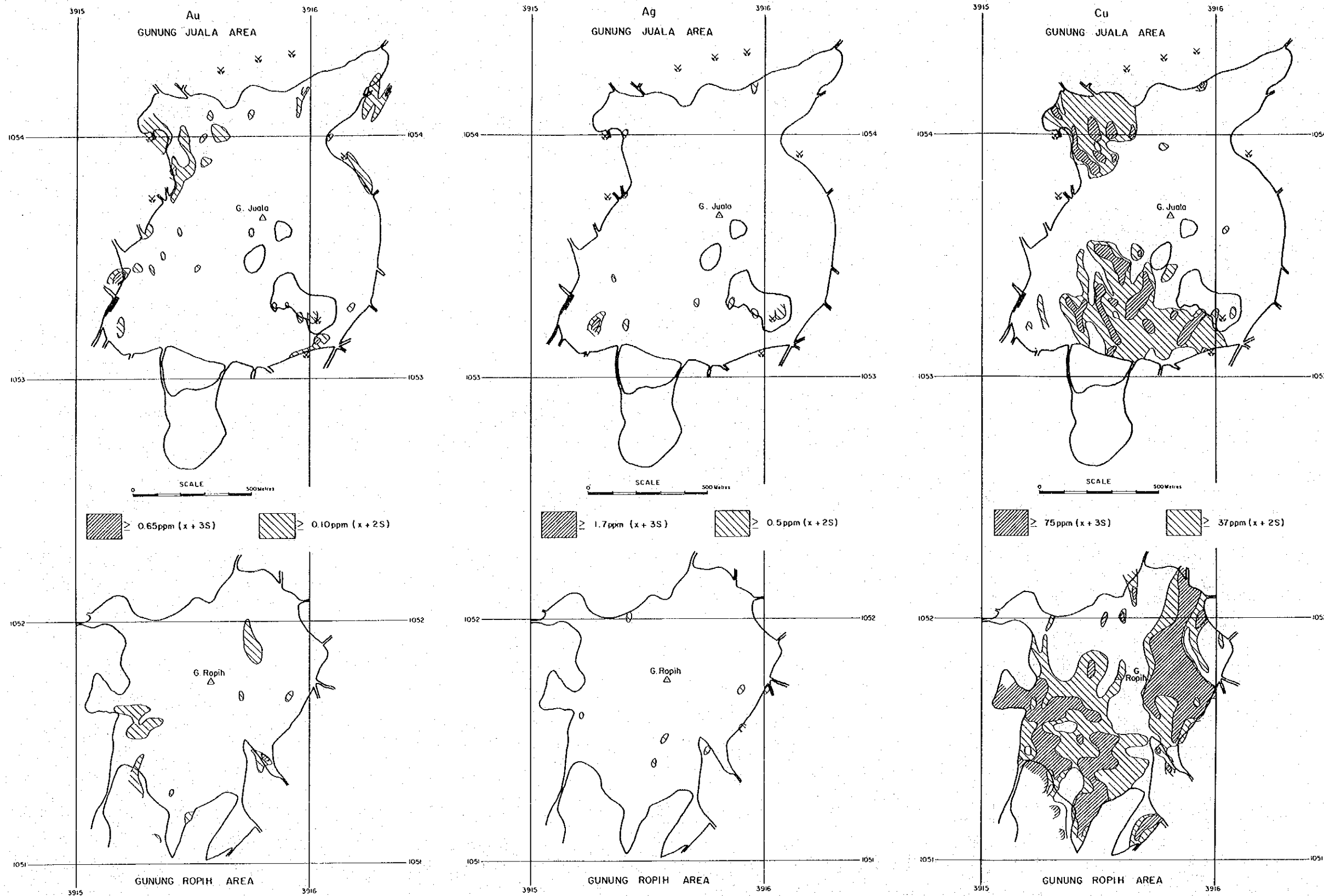
Fig. I -36 Results of Geochemical Soil Survey, Au, Ag and Cu Gunung Ropih-Gunung Juala Area
