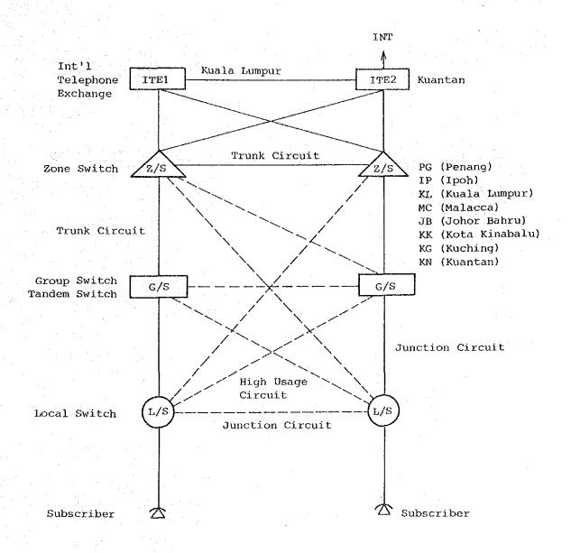
Figure III-2 Telephone Network Configuration in Malaysia
