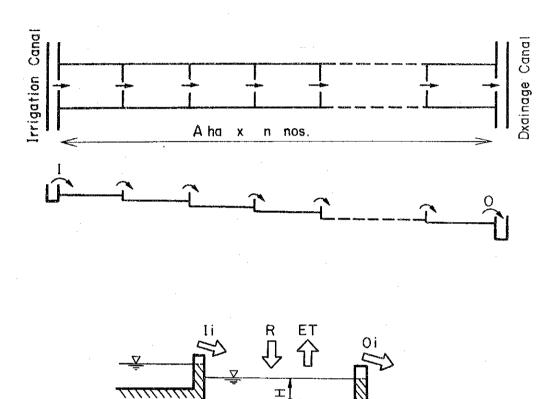
Fig. 9 Plot-to-Plot Irrigation Model
