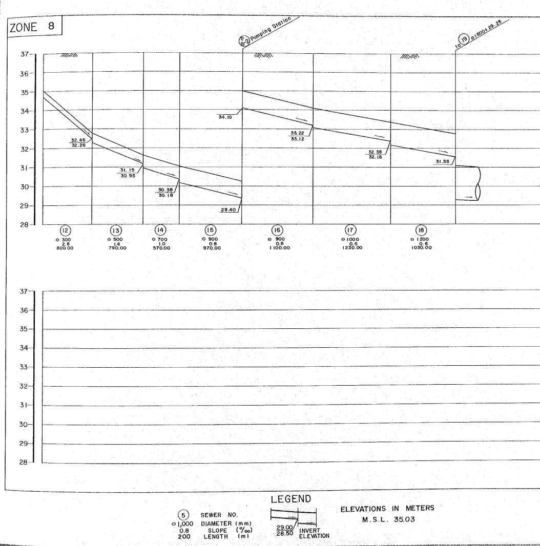
2 - 16 SEWERAGE SYSTEM PROFILE SCALE VERTICAL 1:100 HORIZONTAL 1:30,000
