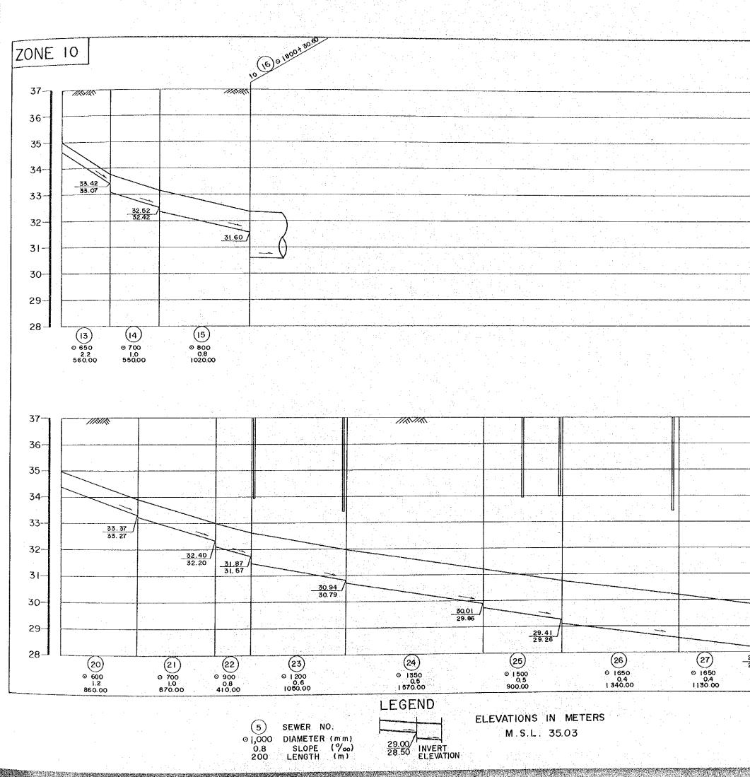
2 - 19 10 38 0 2700 28.76 TINTR 28.27 28.12 28 <sup>©</sup> 1800 0.4 1 150.00 ----27, 66 SEWERAGE SYSTEM PROFILE SCALE VERTICAL 1:100 HORIZONTAL 1:30,000 a gun gana ang
