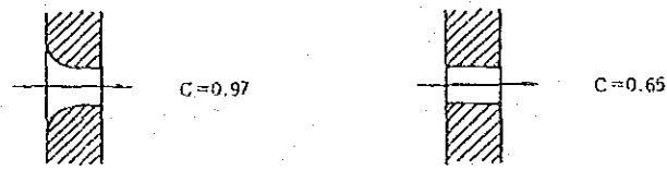
Fig. III-8-37 Shape of orifice and value of discharge coefficient
