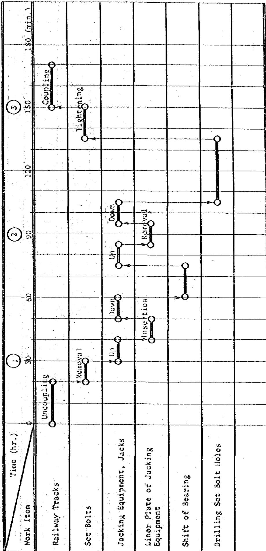
Fig. 3-14 Time Schedule of Anchor Span Shoe Adjustment
