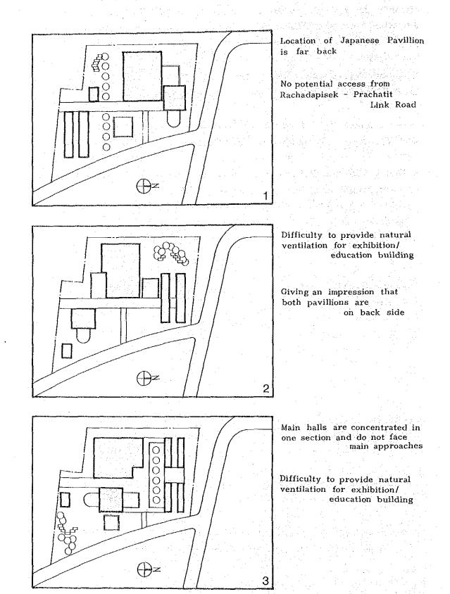
After studying above alternative plans, it was decided that the final site plan, as shown below, which was revised on the basis of plan "l" is to satisfy all basic criteria previously given. Accordingly external space for each building was secured in accordance with each purpose and function.
