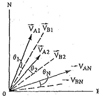
Fig. V-1-7 Wind vectors between station A and station B
