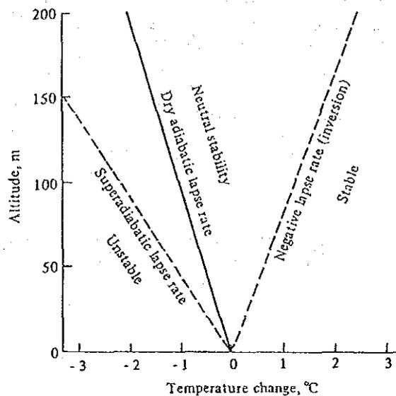
Fig. V-1-11 Atmospheric air-temperature lapse rates
