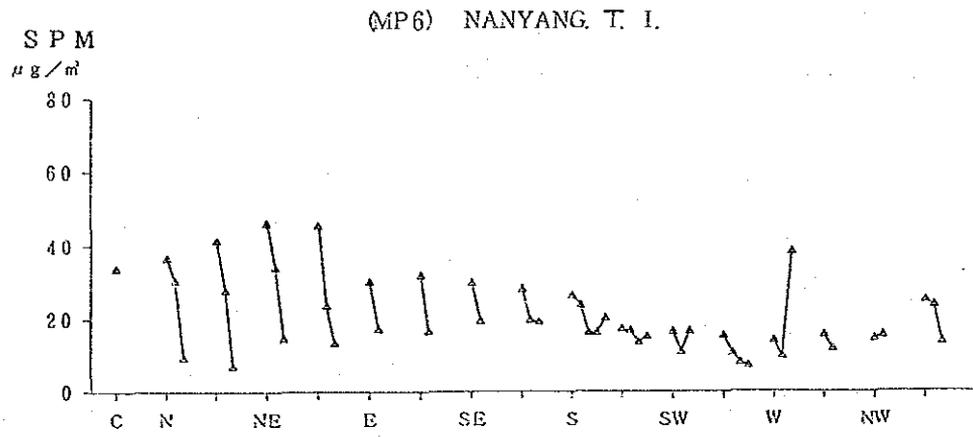
Fig. V-1-23 SPM concentration on wind direction and wind velocity ranks
