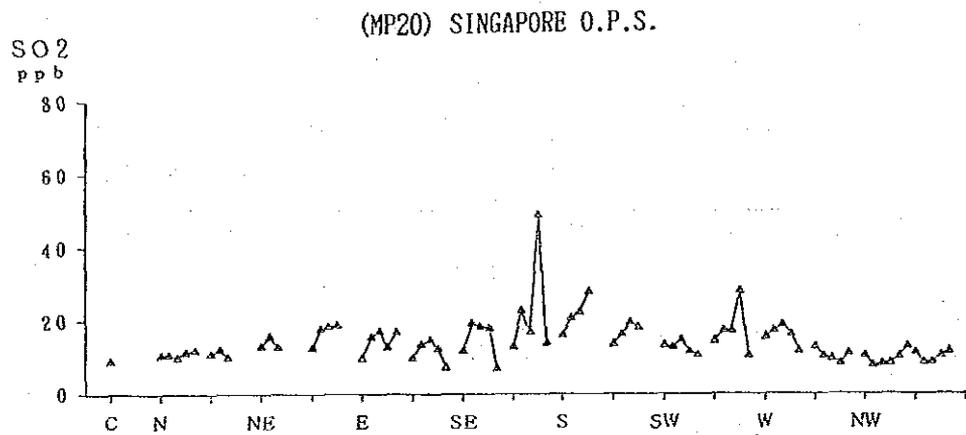
Fig. V-1-18-(2) Average SO<sub>2</sub> concentration for wind direction and velocity ranks
