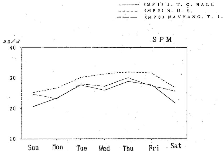
Fig. V-1-21 Weekly variations of SPM concentration by Beta ray dust analysers
