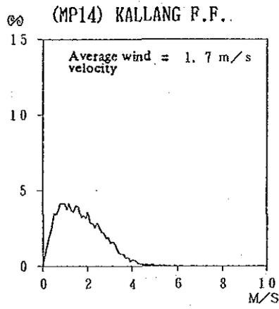
Fig. V-1-5 Frequency distribution of wind velocity
