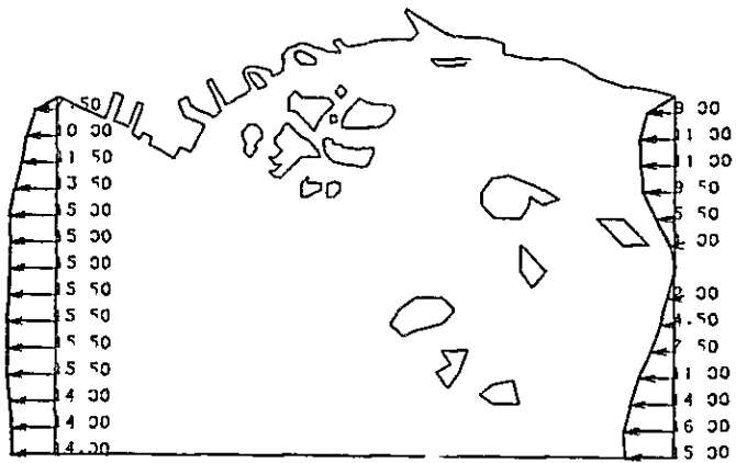
Fig. III-5-10 Velocity distribution on the open boundary (westward current)
