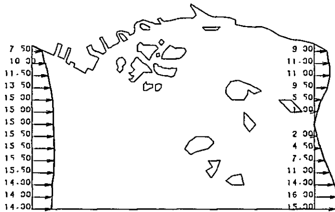
Fig. III-5-11 Velocity distribution on the open boundary (eastward current)
