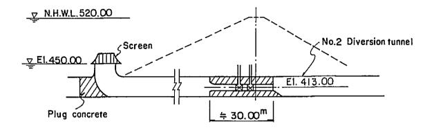
No.2 diversion tunnel will be reused as a river outlet as illustrated above after completion of the dam.
