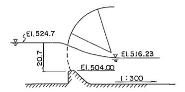
By the hydraulic analysis of non-uniform flow, the water level at immediately downstream of spillway weir is obtained to be El. 513.25 m as mentioned in the water surface studies.
