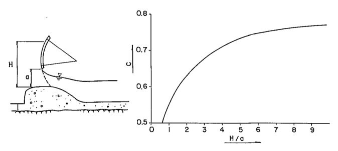
As shown in the above figure, when a F.W.L. is fixed to be 522.00 m, the relation among the opening depth, discharge coefficient and discharge capacity are calculated by the following equations.
