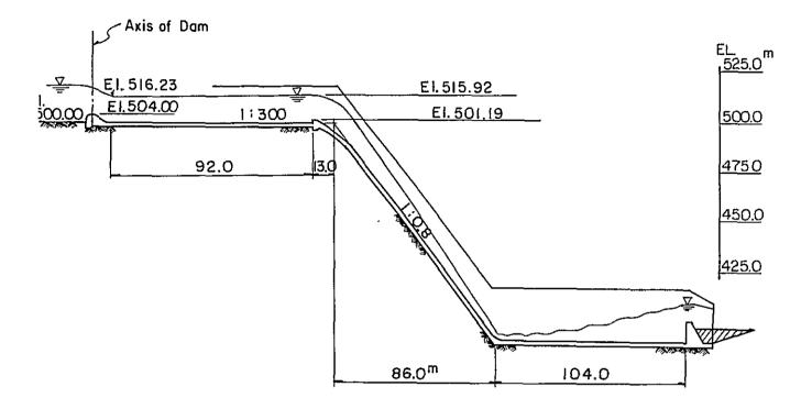
The spillway is of open chute type made of reinforced concrete. The spillway is composed of four parts, i.e., i) gated overflow weir at the beginning near the dam axis, ii) a flat open channel with a gentle slope of 1/300, iii) a steep chuteway with a slope of 1:0.8 and iv) a flat and deep stilling basin ended by a sub-dam. The main dimensions are illustrated in the above drawing.
