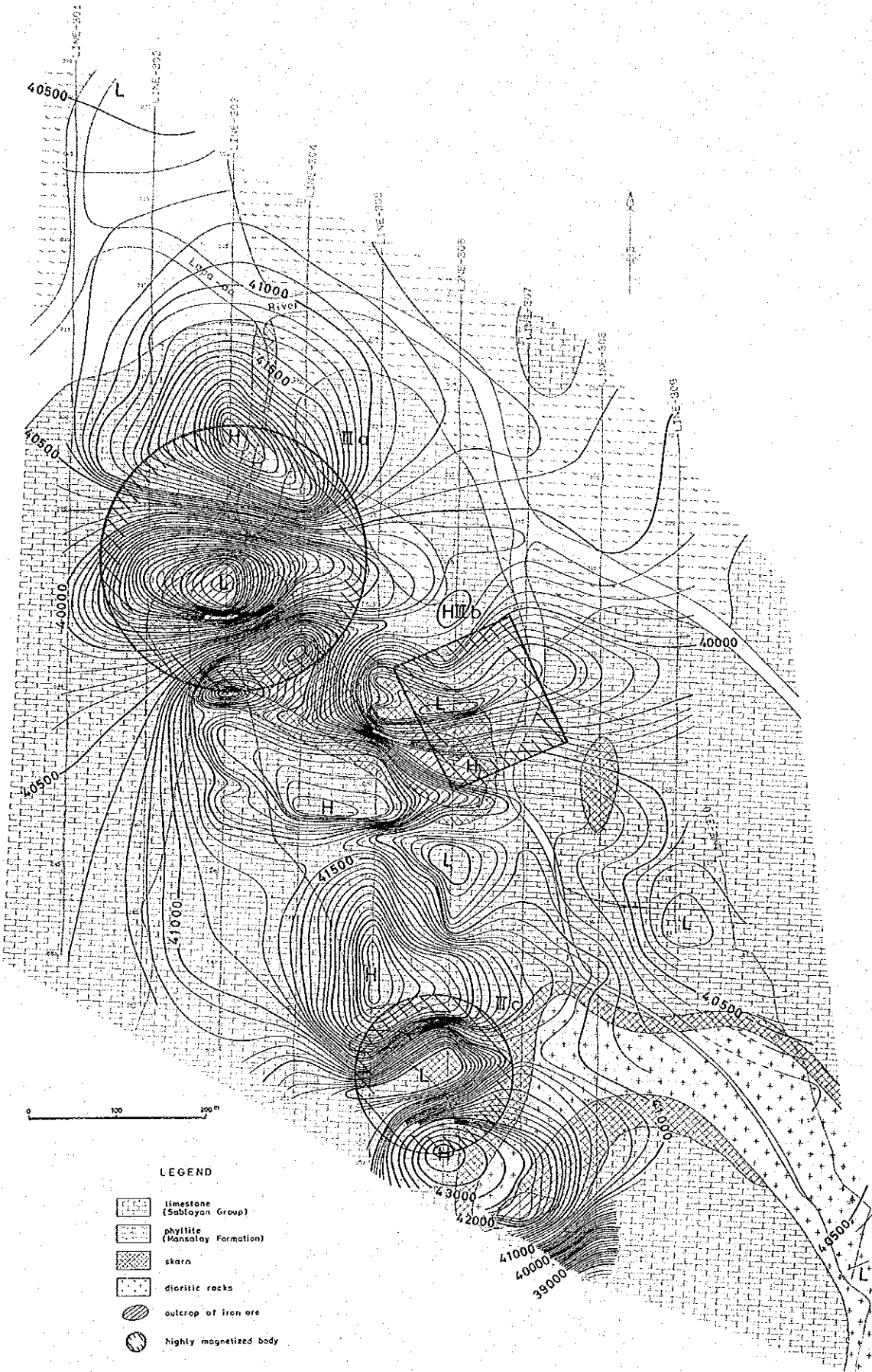
Fig. 18 Interpretation Map of Ground Magnetic Data on Lapa-ao Iron Deposit
