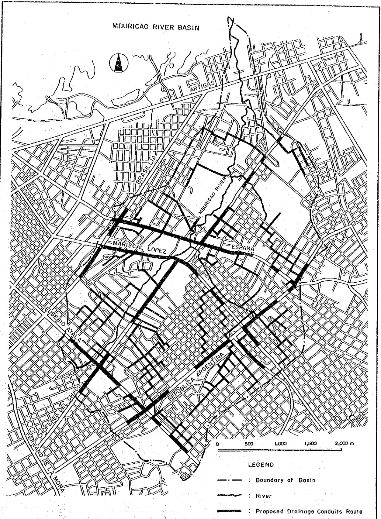
Fig. 7-1(2/2) LAYOUT OF THE DRAINAGE FACILITIES FOR STUDY CASE I FOR MASTER PLAN (MBURICAO RIVER BASIN)
