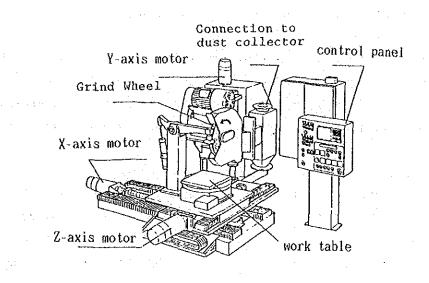
Four-face CNC Automatic Grinding Machine
