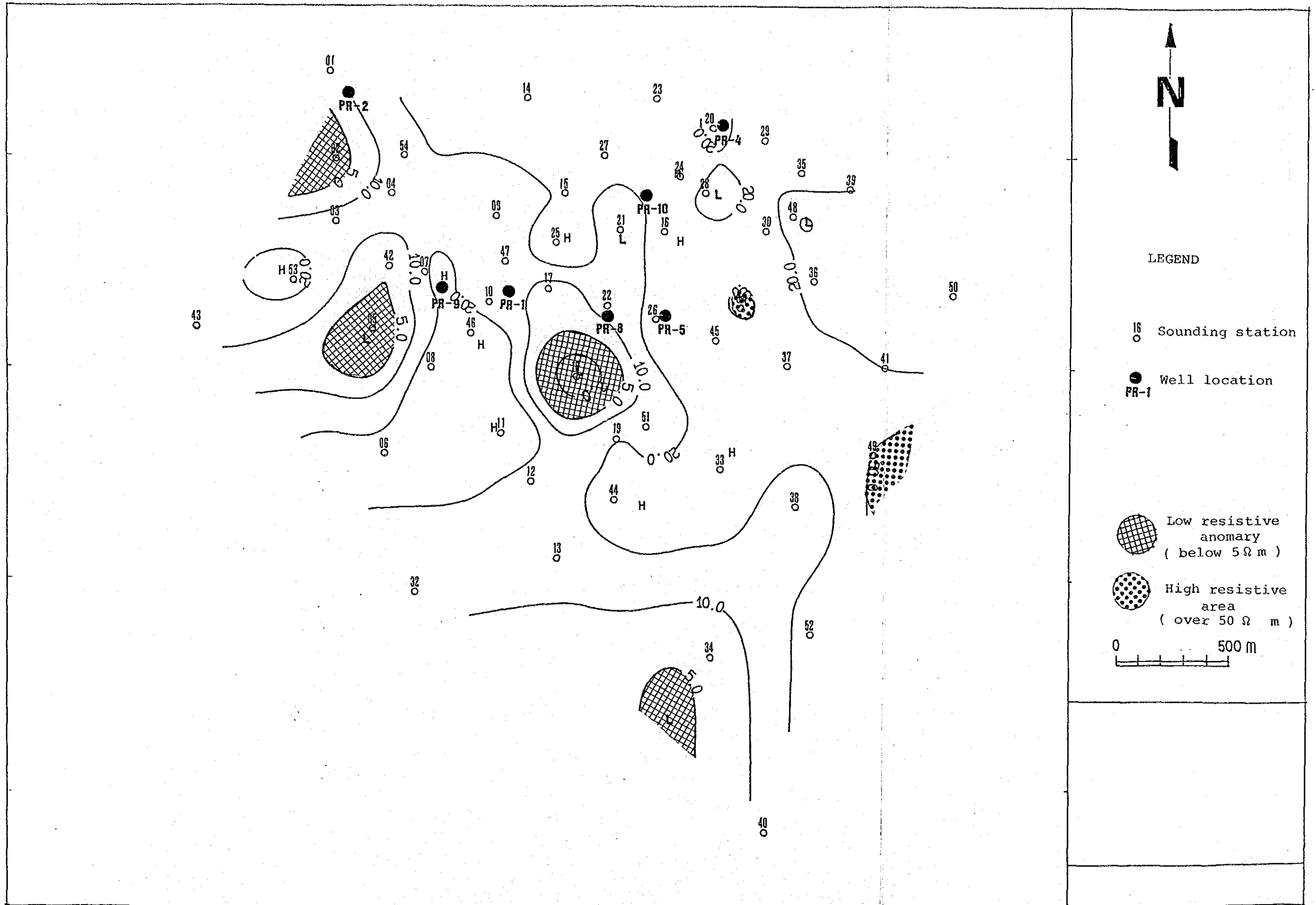
Fig. 33. Resistivity map (TE mode), 500m below sea level
