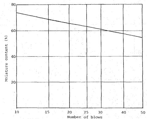
Results. Liquid limit (LL): 63.0 % Plastic limit (PL): 33.0 % Plasticity index (PI): 30.0 % Linear shrinkage:
