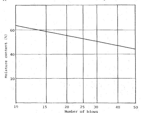
Results. Liquid limit (LL) : 53.0% Plastic limit (PL): 30.0% Plasticity index (PI) : 23.0% Linear shrinkage : 10.0%
