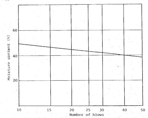
Results. Liquid limit (LL): 43.0 Plastic limit (PL): 30.0 Plasticity index (PI): 13% Linear shrinkage:
