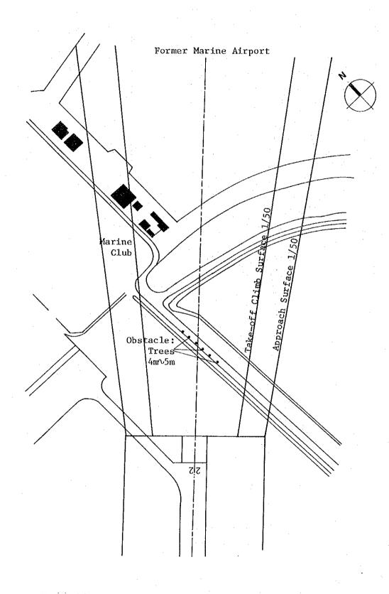
Fig. 5.3.1 (2) Obstacles in Final Segment of Approach Area for Runway 22
