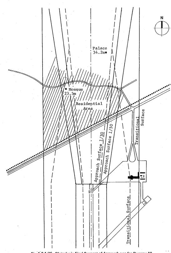
Fig. 5.3.1 (3) Obstacles in Final Segment of Approach area for Runway 18
