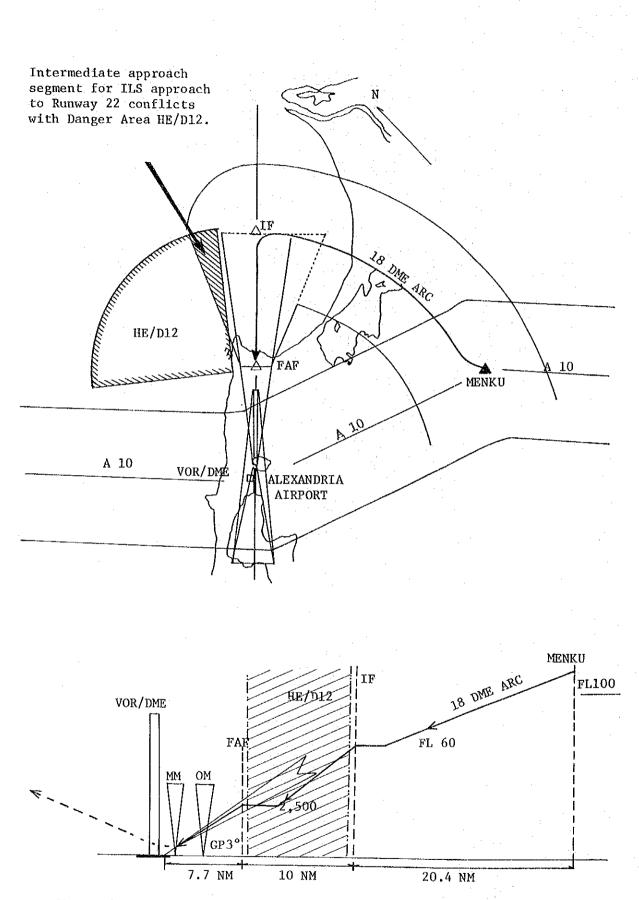
Fig. 6.4.2 Relations between Danger Area HE/D12 and Intermediate Segment for ILS Approach to Runway 22
