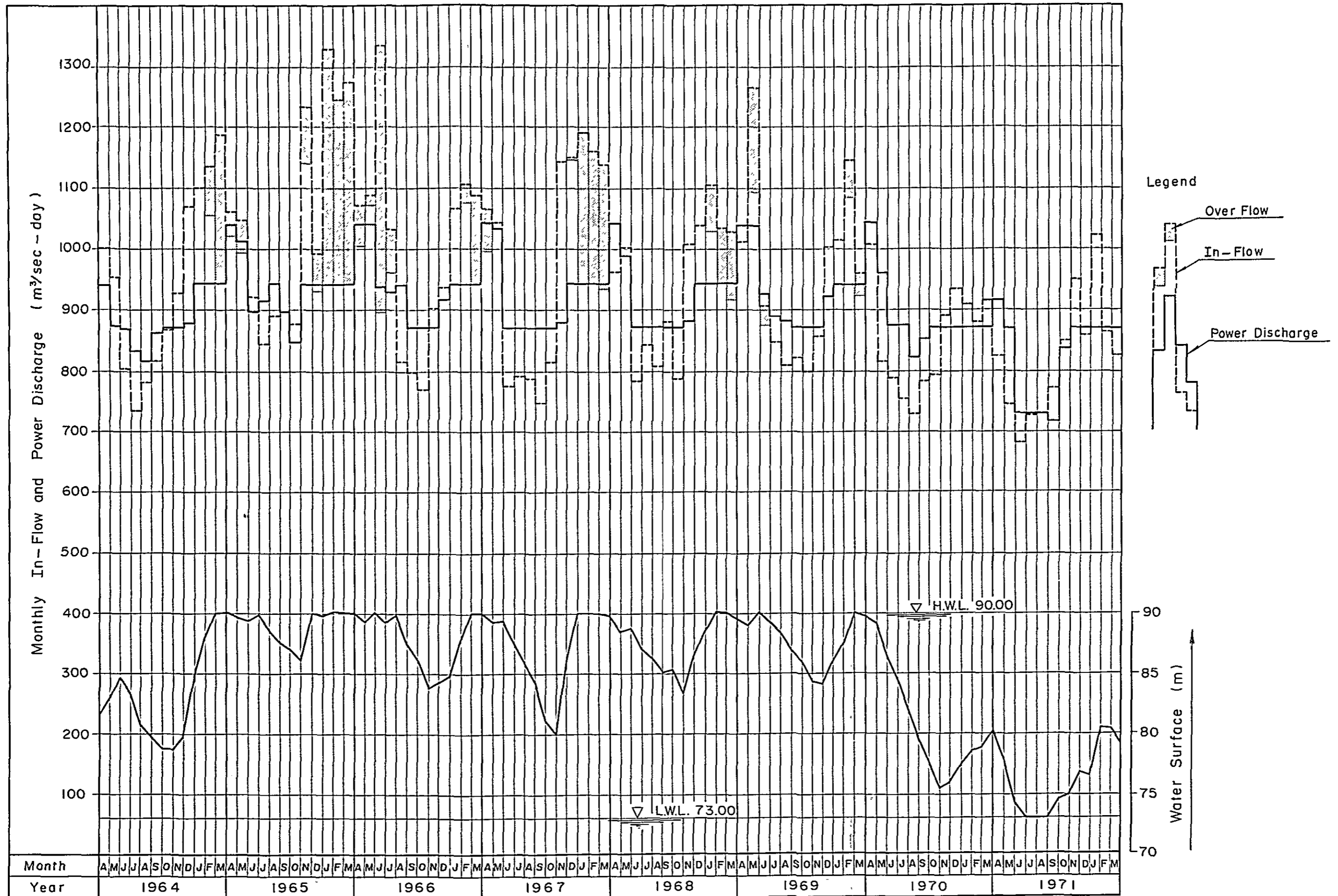
Fig.-9.6 In-Flow Power Discharge and Reservoir Water Surface of Salton Gorge Power Station
