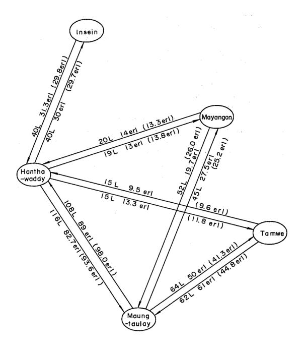
Fig. II. I. I. I Junction Traffic Flow Diagram of Rangoon Network. (Present)
