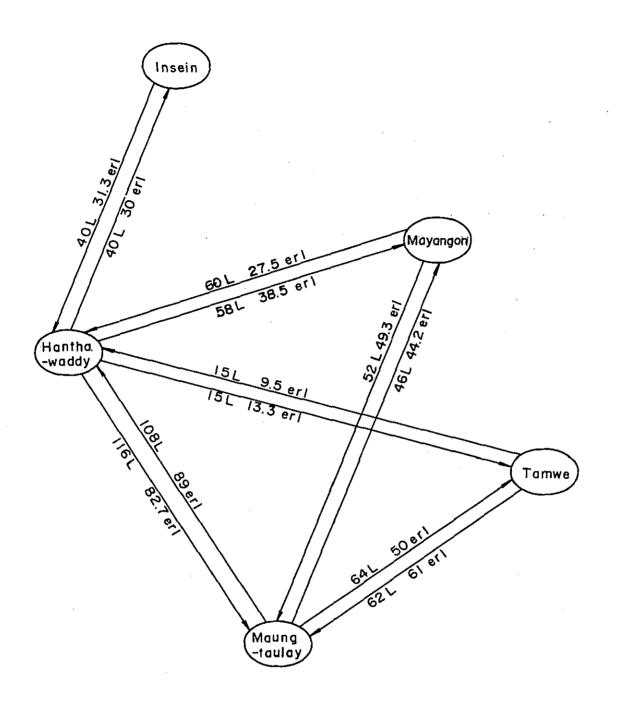
Fig. I.I.I.2.(1/2) Junction Traffic Flow Diagram of Rangoon Network (Before World Bank Project)
