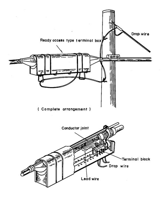
Arrangement inside ready access terminal box (Example of drop:wire from aerial cable ready access terminal box)
