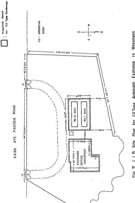
Fig. TL. I. I. 5 Site Plan for C2Type Automatic Exchange in Mayangon
