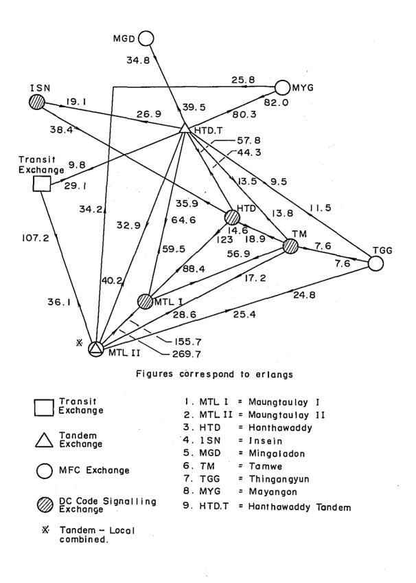
Fig. II. I. 2 (<sup>2</sup>/2) Junction Traffic Flow Diagram of Rangoon Network (After World Bank Project)
