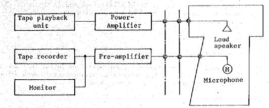
Circuit newly provided in this auditorium shall be used for the microphone and the loud speaker. If no existing circuits are available for this purpose, cables similar to cabtyre cable shall be used for connection.
