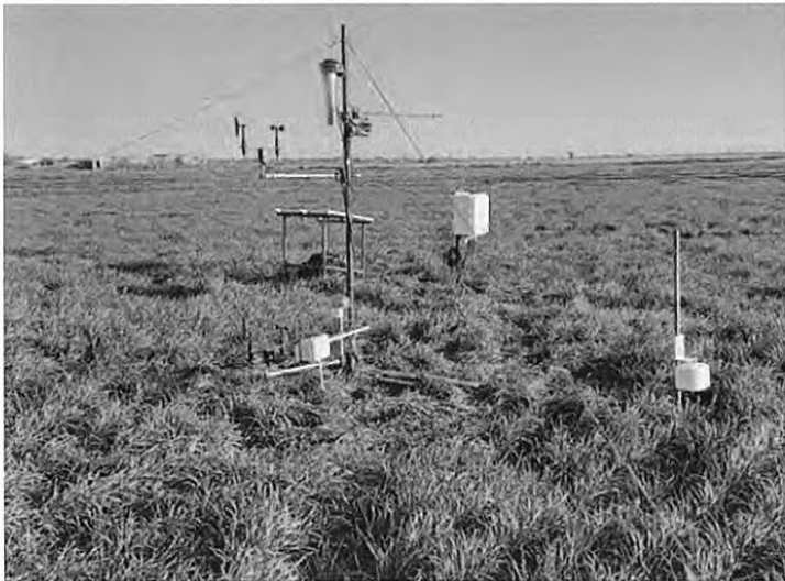
Weather station for monitoring microclimate in wheat field
