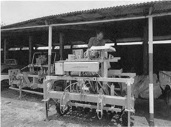
Precise plot drill for research purpose
