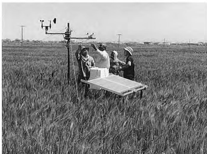
Mobile weather station for microclimate monitoring in wheat fields
