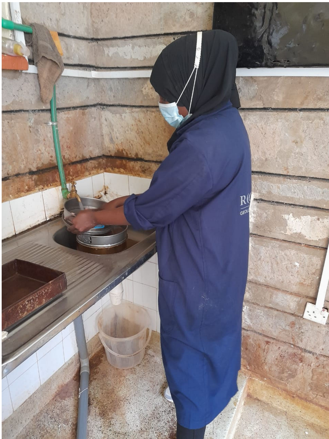
Wet sieving of soil samples
