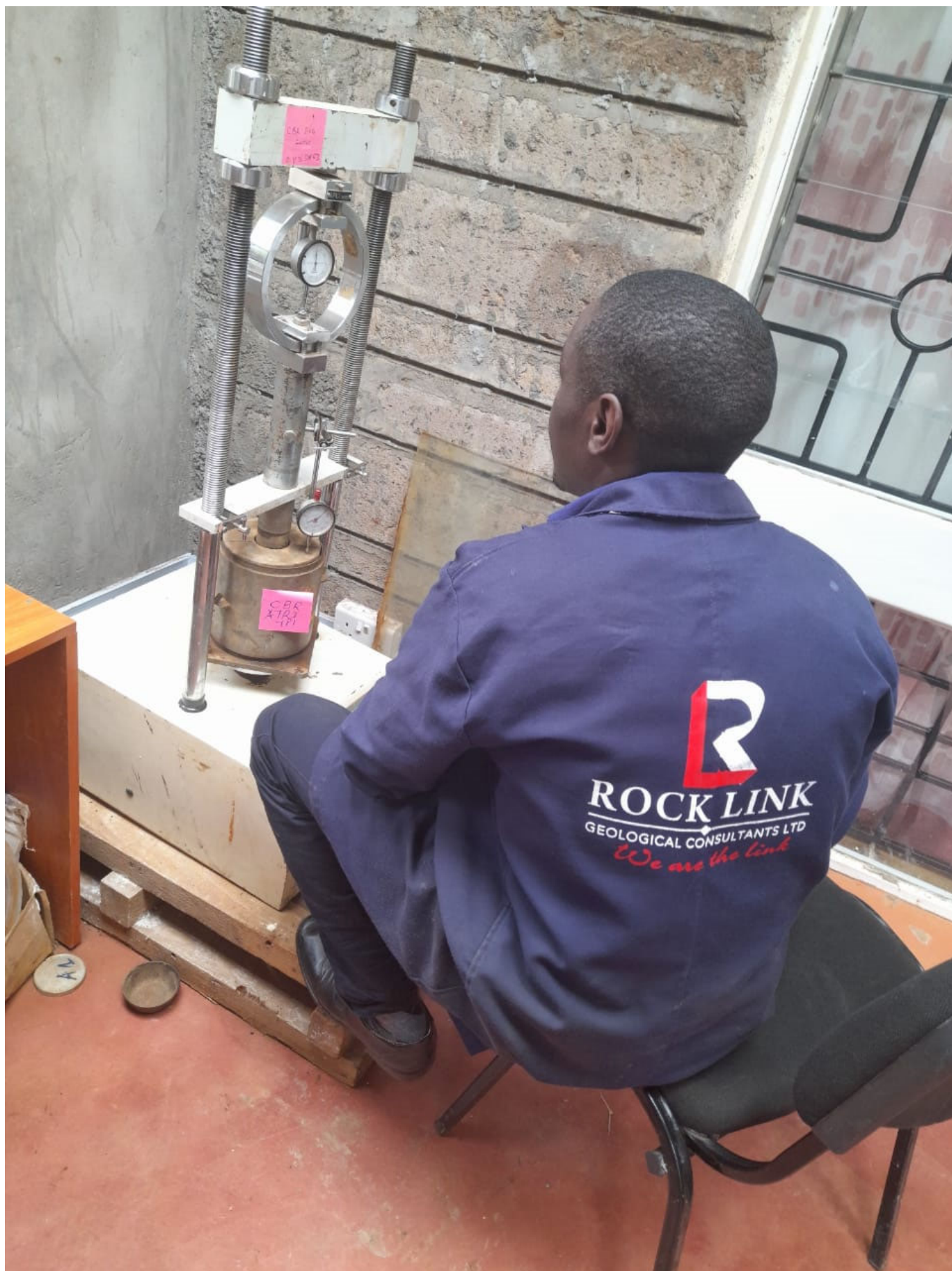
CBR test in progress
