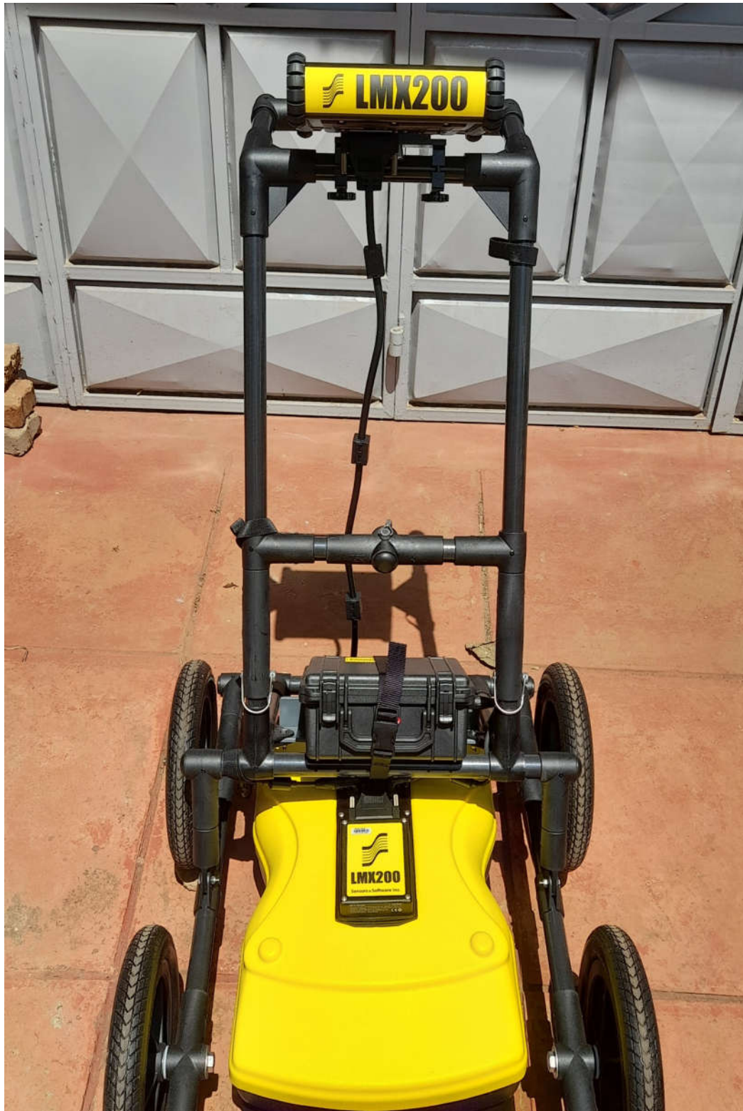
Figure 5-Radar Scan Survey Machine(LMX200)
