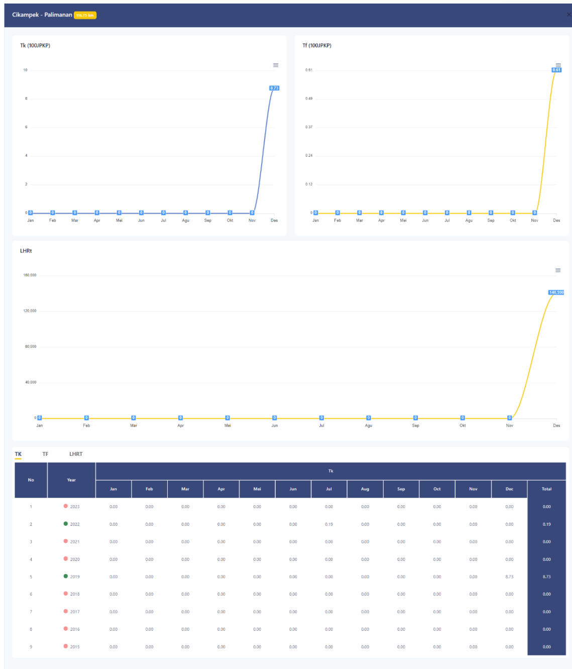
Figure 4.26 User Interface Design for "Accident Rate" and "Fatality Rate" analysis
