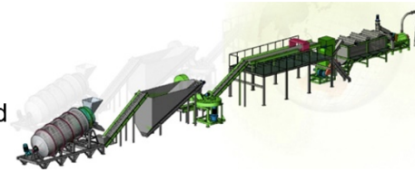
Production line of recycled PET pellets
