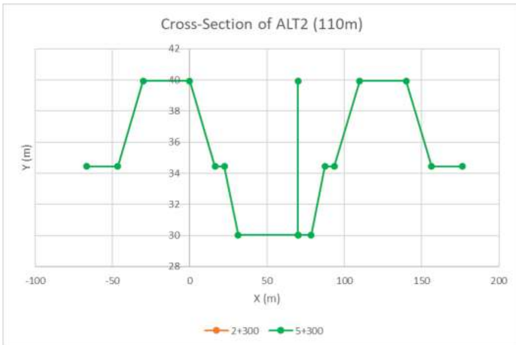
Figure 4.6.42 Cross-Sectional View of Widening of the Existing Waterways (Aral Tail and RBOD-II) (ALT2)
