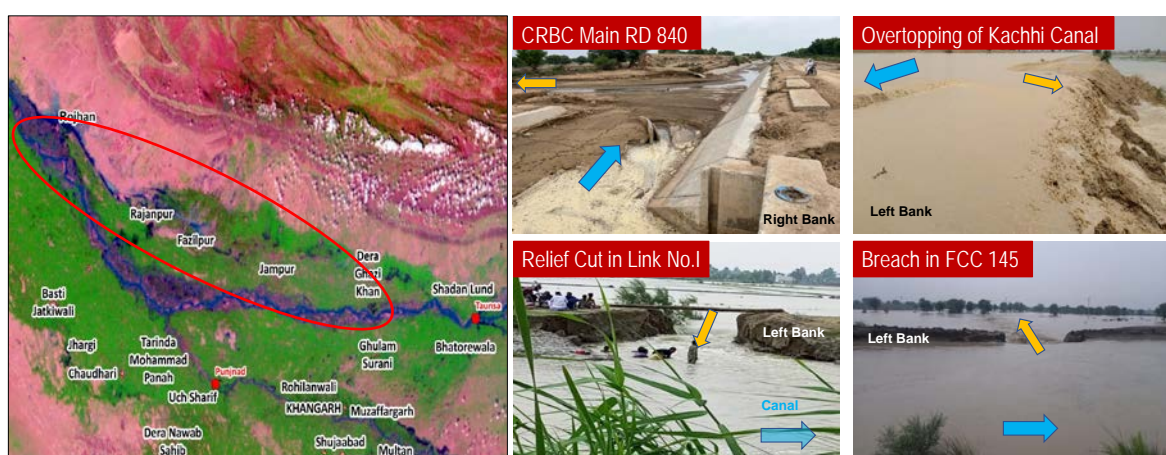
Figure 2.4.11 Damage of Facilities in D. G. Khan Irrigation Zone during the 2022 Flood
