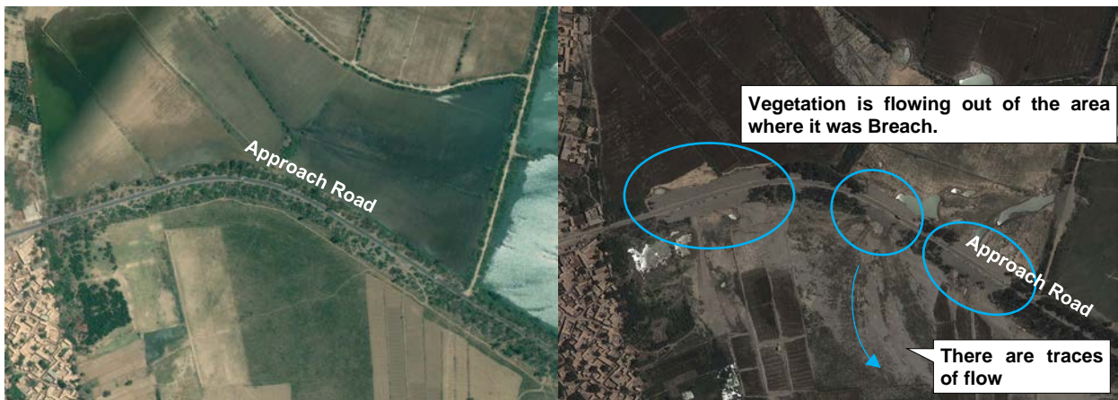
Figure 2.2.14 Conditions before and after the 2010 flood at the Breach site in Jinnah Barrage
