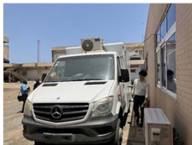
X-ray Inspection Equipment (Mobile-type) (Out of Order)
