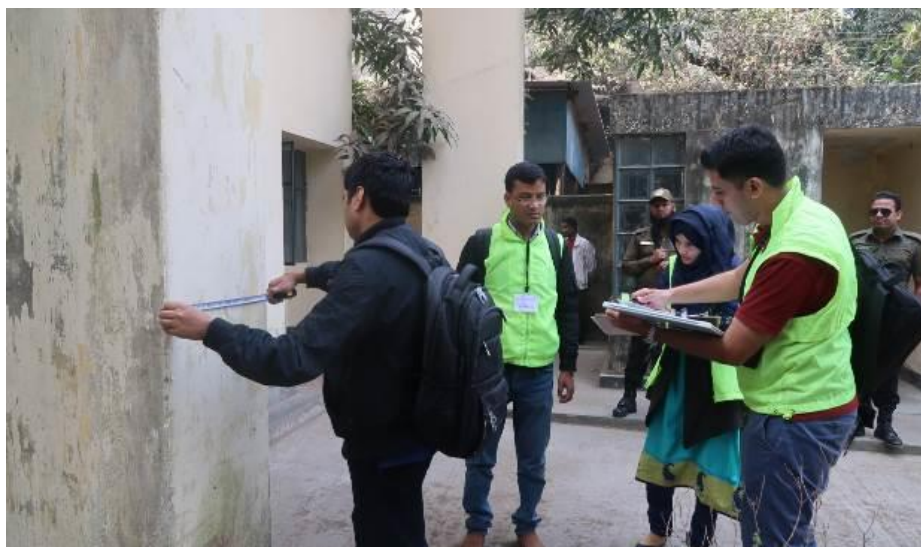
Pic. 6 Building survey to make as-built drawings
