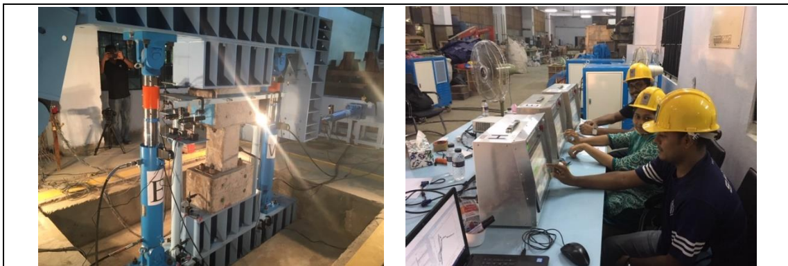
Pic.1 Column tests at BUET (provided jack systems, measurement systems, member specimens, reaction frames are under use) (July-December 2018).
