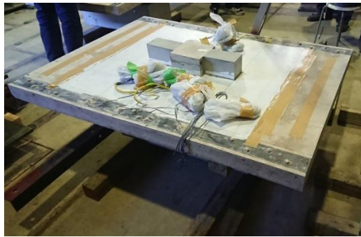
Pic. 23 Flat plate specimen with wing wall tested in DaidoU
