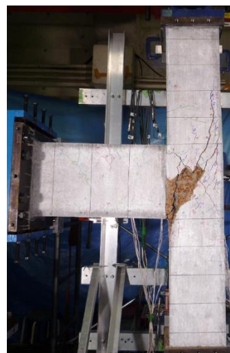
Pic.13 Pull-out failure of beam longitudinal bar
