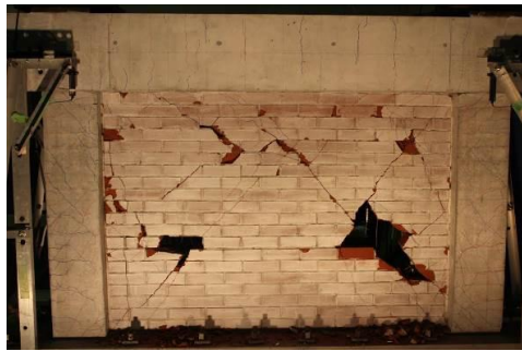
Pic.8 Failure pattern of a specimen tested by TohokuU in Japan (2016)
