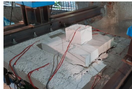
Fig. 31 A flat plate specimen retrofitted with smaller drop panel and its load-deflection curve tested in HBRI.
