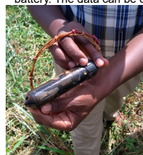
HOBO Data Logger with sensor cable at RGS 4BE01 Maragua
