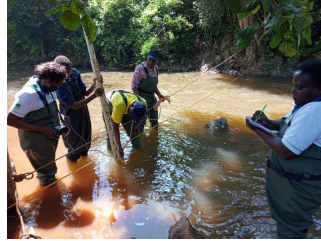
Discharge measurement at RGS 4DC03 Rupingazi on December 9, 2022 using propeller type current meter.
