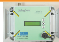
1. Open the plastic cover on both sides and loosen all four screws
