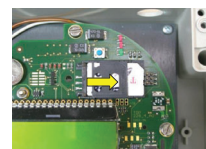
5. Press the SIM card holder down and push the fastener back in place
