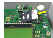
4. Insert or remove the SIM card as illustrated
