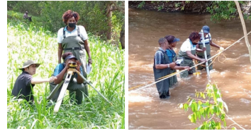
←River cross section survey and discharge measurement at RGS 4AC03 Sagana on December 19, 2022
