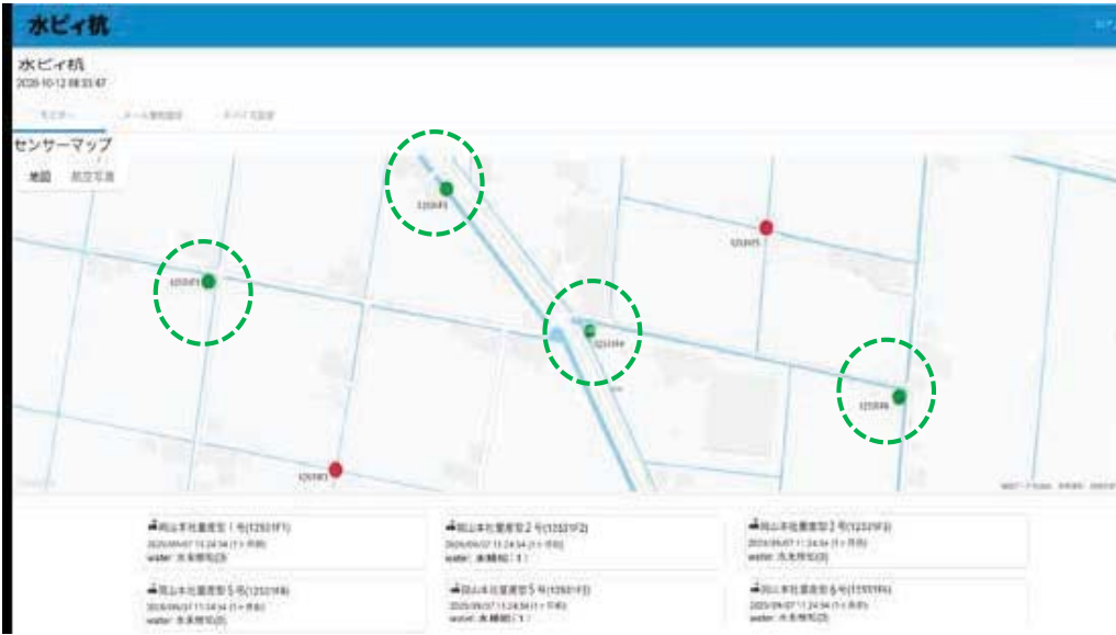
Monitoring of flood detection with GIS application- green color denote the sensor to detect the flood.
