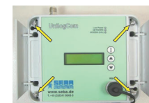
6. Put the cover back on, tighten the screws and close the device
