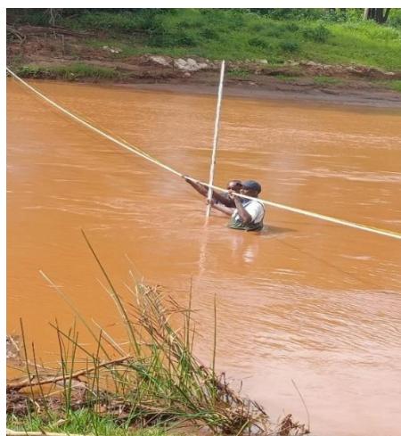
Photo 4: Mr. Masika and a local volunteer wading through the river during the cross-section survey at Kathita 4F10
