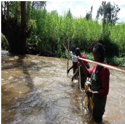
Photo 3: Ms. Doreen, Ms. Jane (SWO, Upper Tana sub-basin) and Dr. Masika carrying out discharge measurement at 4AC03
