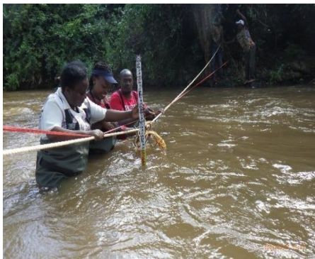
Photo 4: Dr. Masika, Ms. Doreen and Ms. Jane (SWO Thiba Sub-basin) during discharge measurement at 4DC03
