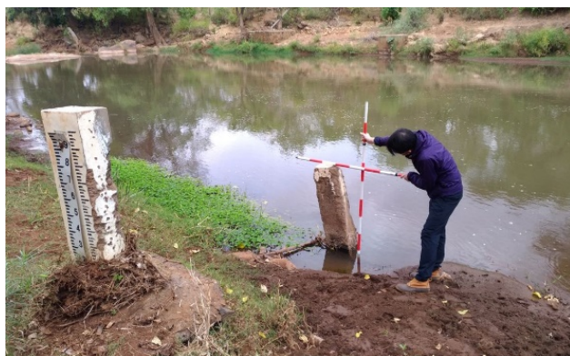
Candidate Gauging Station for Discharge Measurement Practices, 4F10 Kathita in Meru SBO. The first staff gauge is slightly leaning. (2021/7/8)
