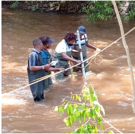
Photo 6: Discharge measurement in progress using the propeller- type current meter at Sagana 4AC03
