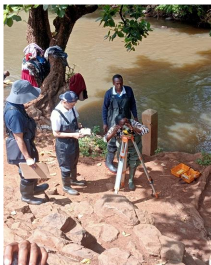
Photo 3: Ms. Jane Njuguna taking readings during cross-section survey at 4DC03 Rupingazi.
