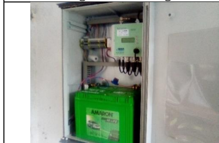
2. SEBA Data Logger in station 4DA11(Thiba). 2&3Newly Installed Telemetric Meteorological station and staff gauge outside Murang'a Sub-Regional Office
