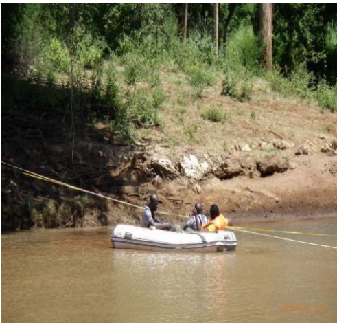
Photo 2: Dr. Masika and Mr. Gordon using the propeller-type current meter during discharge measurement while Ms. Doreen taking the bookings at 4F10
