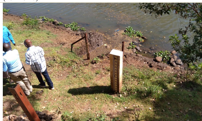
Site Reconnaissance to Regular Gauging Station 4DD02 Thiba. The 1 st and the 2 nd Staff Gauges. (2023/1/25)
