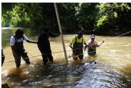
Photo 2: Mr. Masika illustrating the use of a propeller-type current meter during discharge measurement at 4DC03
