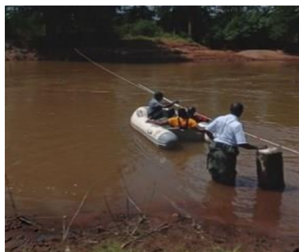
Photo 6: Mr. Gordon, Ms. Doreen, and Dr. Masika carrying out discharge measurement using a propeller-type current meter in a boat at 4F10.
