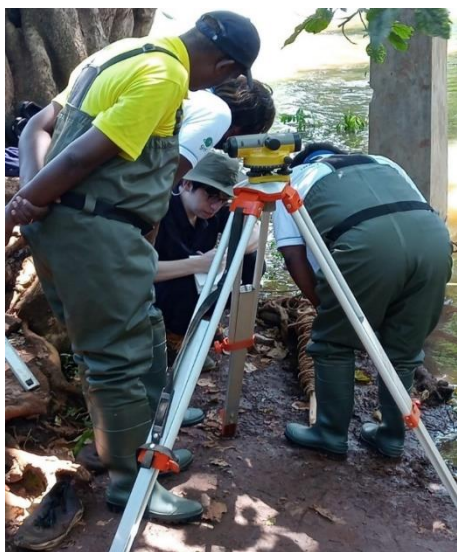
Photo 1: Mr. Kato explaining the principle of leveling at the Rupingazi station 4DC03 during the river cross-sectional survey
