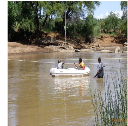
Photo 1: Dr. Masika, Ms. Doreen, and Mr. Gordon carrying out the cross-sectional survey at 4F10 using a boat
