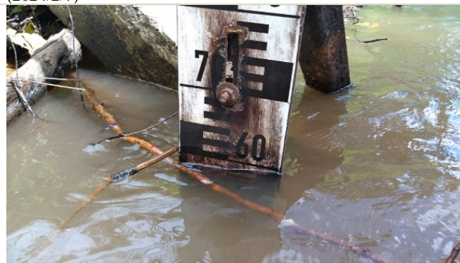
Exercises of Discharge Measurement at 4AC03 Sagana. The Water Level at 0.59 m. (2024/2/7)
