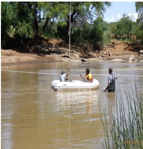
Photo 1: Dr. Masika, Ms. Doreen, and Mr. Gordon carrying out the cross-sectional survey at 4F10 using a boat
