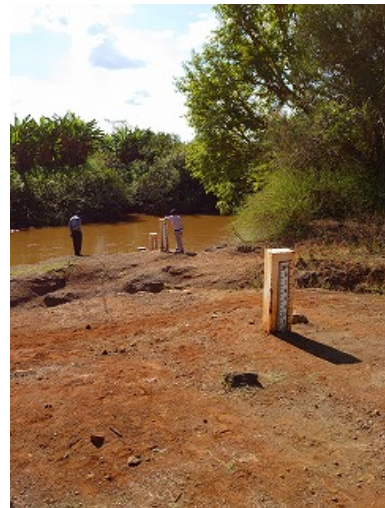
Telemetry Station in Tana Basin, 4BE10 Tana Rukanga. 4BE10 Tana Rukanga. Staff Gages located in the left bank (2021/10/26)
