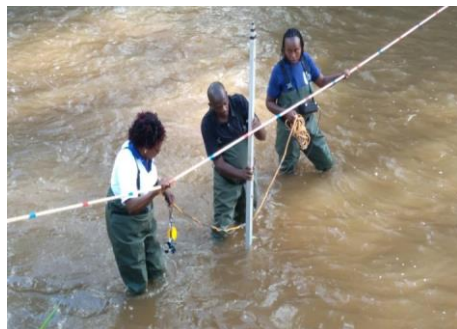
Photo 2: Ms. Jane Wairimu Njoroge, Ms. Doreen and Dr. Masika carrying out discharge measurement at 4AC03.
