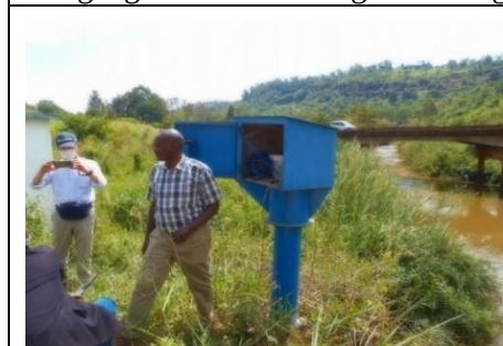
3. The housing structure of HOB0 data logger in 4BE01(Maragua) 2. Checking of the equipment 3. Faith demonstrates data reading from the logger to the PC through the coupler.
