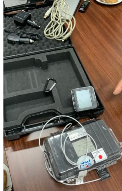
Image 4 Dynamic Response Intelligent Monitoring System (DRIMS) provided under the road maintenance component. Used by the MPW-BARMM for measuring road roughness. The condition is good, and it is easy to transport. (source: Photographed by the ex-post evaluator)
