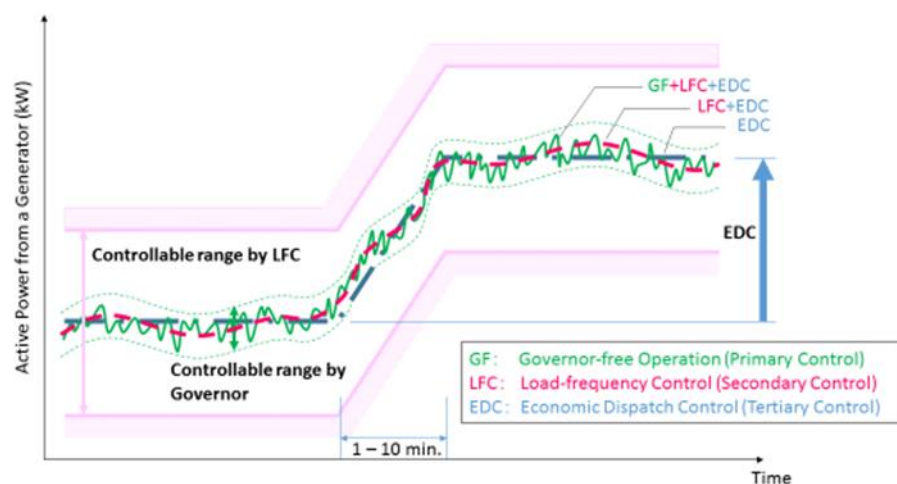
Figure 1-3 Basic idea of frequency control
