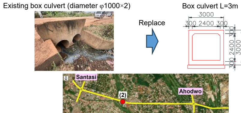
Figure 2-12 Structure (2): Box Culvert L=3m
