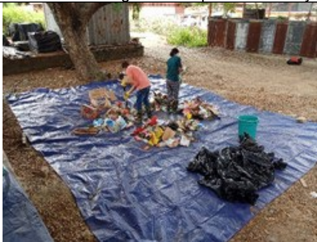
Sampling by Quartering Method for Waste Among and Composition Survey
