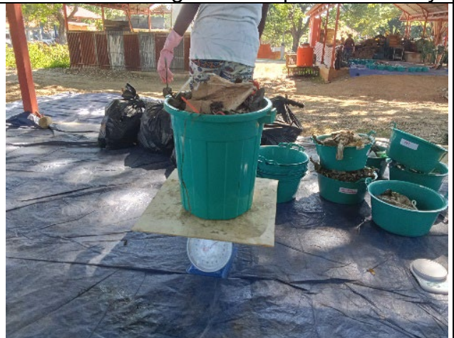
Measurement of Bulk Density for Waste Among and Composition Survey
