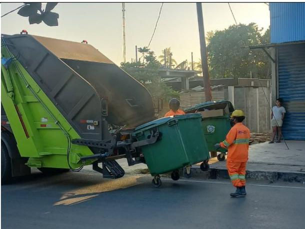
Waste Collection Activity with Newly Introduced Waste Collection Vehicle (Compactor Vehicle) No.1
